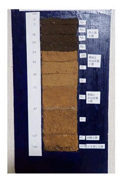
Lack film method for soil monolith preparation as carried out by K. Tsutsuki
